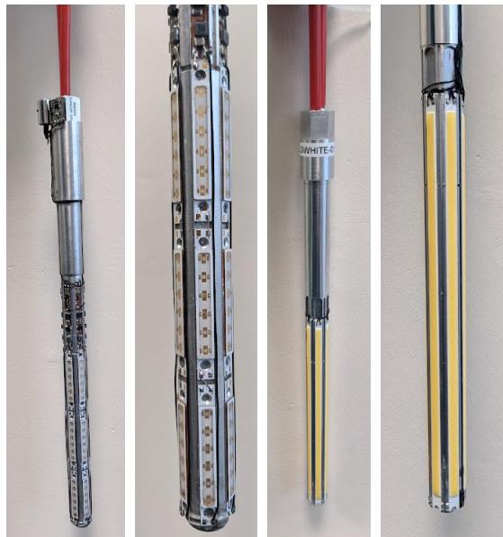
Figure 2.7: Left two images: First-generation PhotoLED with a  $\lambda_{\text{max}}$  emission of 424 nm. Right two images: Second-generation PhotoLED, white light emission is generated through the use of blue LED strips coated in yellow phosphor. The two red tubes at the top of the housing are the inlet and outlet for the interior cooling.
