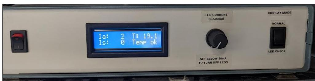
Figure 2.8. Second generation control box for the PhotoLED. In normal display mode the LED current can be set ( $I_s$ ) up to 500 mA. The LEDs turn on once a current of 50 mA has been set. The actual current ( $I_a$ , highest current through an individual strip) can be observed, along with the temperature of the PhotoLED.
