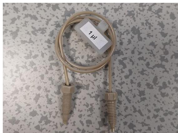
Figure 5.23 PEEK Vici® 1 $\mu$ L sample loop with PEEK end fittings. The length of the 1 $\mu$ L sample loop is far longer than that of the 5 $\mu$ L, the corresponding bore diameter is therefore significantly smaller for the 1 $\mu$ L volume, hence the increased pressure in the system.
