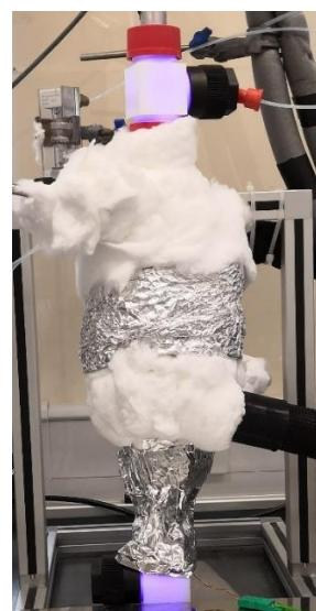
Figure 2.15. Photo of the HPR during low-temperature testing with the PhotoLED *in situ*. There was a need for a high level of insulation to achieve low internal reactor temperatures.
